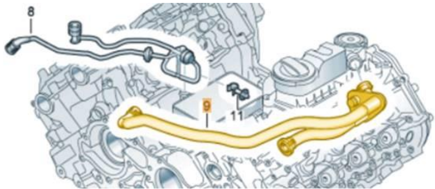
Figure 1. Breather line that needs to be replaced.
