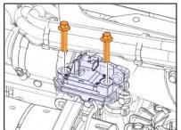
9. Remove the pressure sensor.
