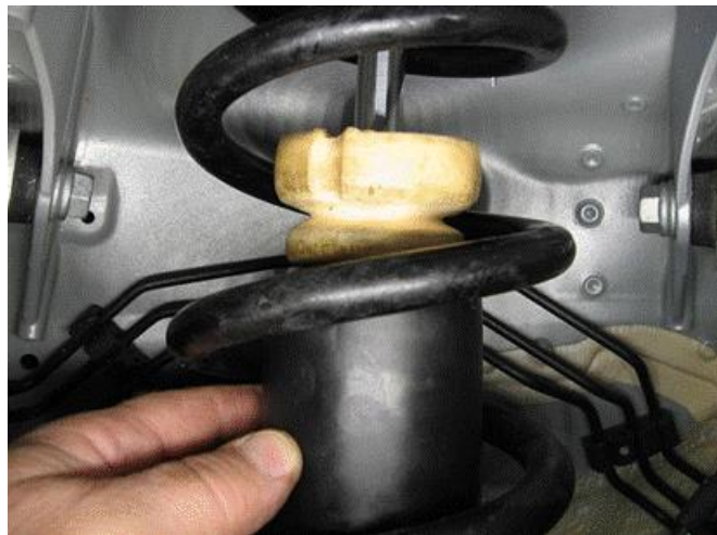
Figure 1. The shock absorbers are sitting incorrectly.
