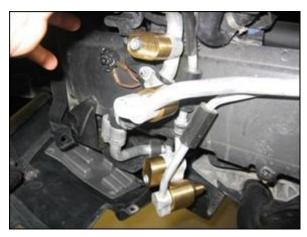
1. Separate the front and rear air conditioning systems for individual rinse operations (Figure 7).
