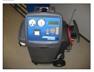
**Figure 1.** The ROB134APF Air Conditioning Service System with VAS 6337/1A Air Conditioning System Flushing Device.
