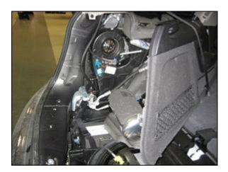
2. Bypass the rear expansion valve with an adapter (Figure 8).
