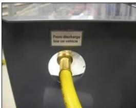
**Figure 2.** Example of a flushing attachment port.
