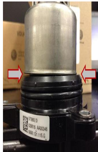
Figure 1. Gap between chamber and seal.
