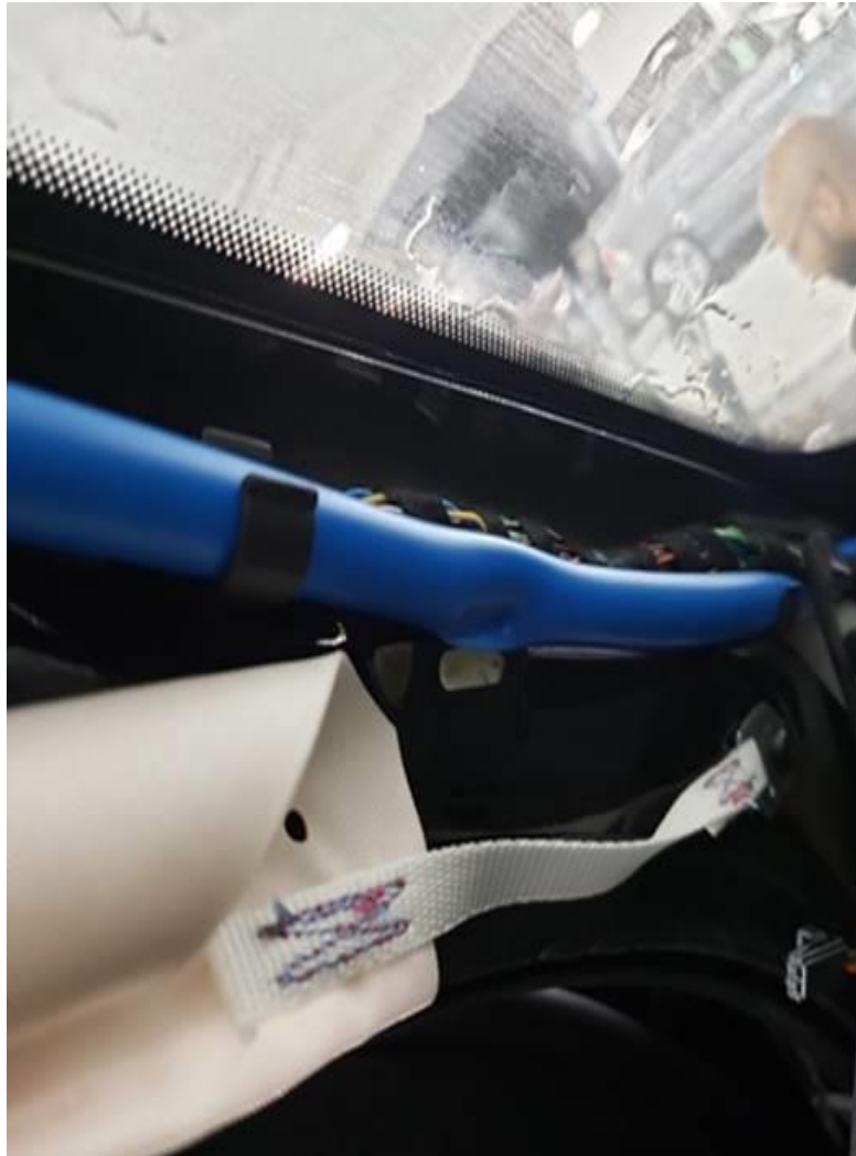
Figure 2. Sunroof drain hose pinched by pillar trim.
