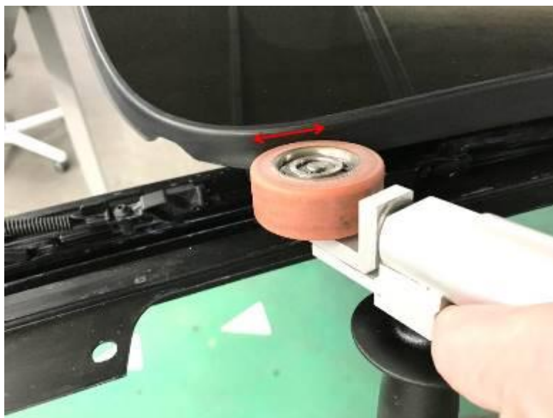
Figure 16. Applying pressure to bonded area with 3356 roller (or equivalent).
