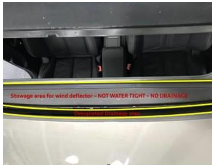
Figure 6. Areas of sunroof opening water elimination capabilities.
