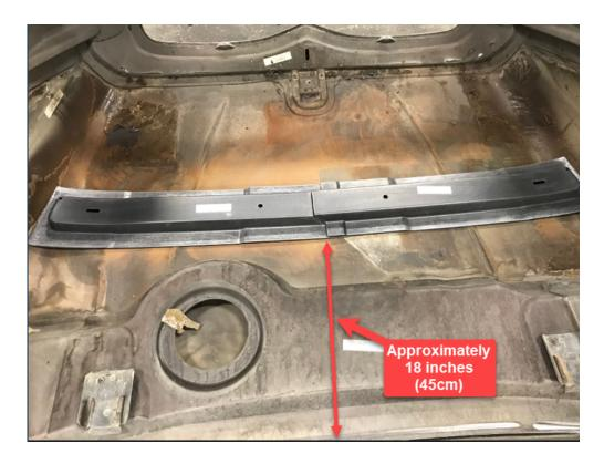
**3.** Notch each of the support sections where they passes over the grooved sections on each side of the hood. One groove and the areas to be trimmed out around it are shown in the photo below:
