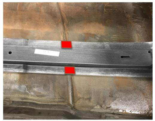
**4.** Install the new hood support using Lord Fusor® T21 Composite Adhesive. Add weight evenally across the new hood support to hold it firmly to the hood. Cure time is 4 hours.
