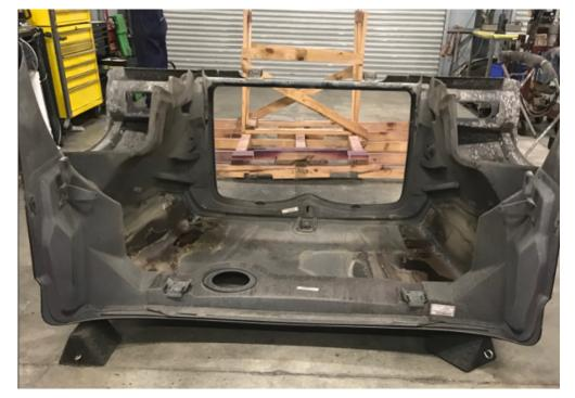
**2.** The new supports should be positioned approximately 18 inches (45 cm) from the rear edge of the hood.
