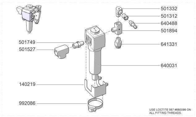
FIGURE 4: FITTING ARRANGEMENT (TYPICAL). ORIENTATION MAY VARY BY MODEL.
