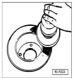
Remove remaining corrosion protection coating or surface rust as follows:
