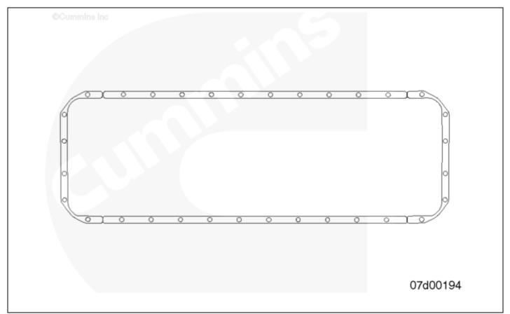
The oil pan full perimeter clamping plates, can **only** be used on engines equipped with stamped steel oil pan options with a single gasket mounting. The oil pan full perimeter clamping plates can **not** be used on oil pans made of materials other than stamped steel, and can **not** be used on oil pan options that use RTV, bedplates, or isolated gasket systems. The oil pan full parameter clamping plates are to be installed on the outside of the rail of the oil pan.
