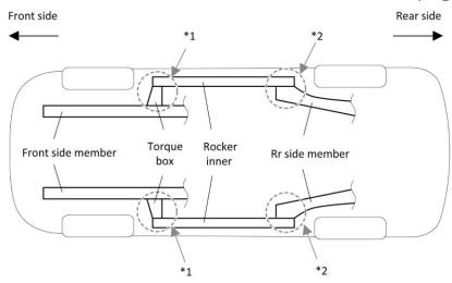
\*1 Torque box hole or Rocker inner hole | \*2 | Rr side member hole or Rocker inner hole
