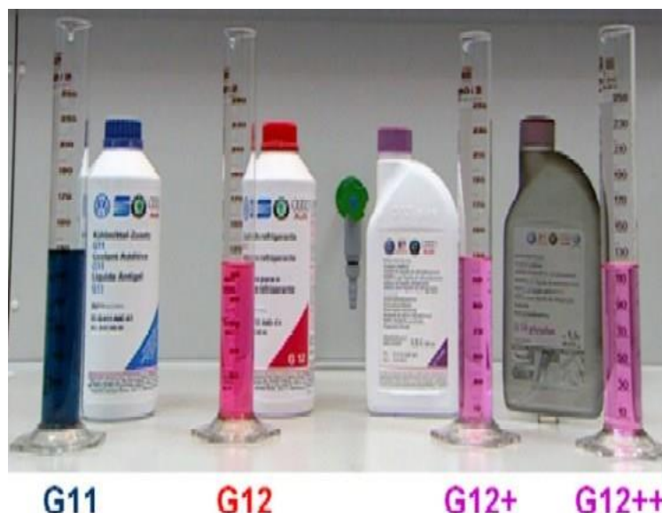
Figure 1. The color of each type of engine coolant. G11 (green-blue), G12 (red), G12+, G12++, G12evo, and G13 (purple).
