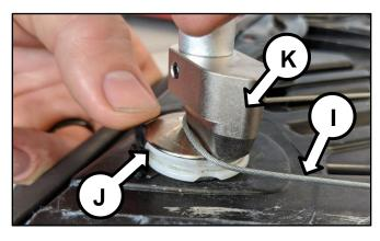
13. Turn the SST (K) clockwise to loop the wire cable (I) onto the pulley (J).
