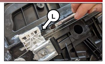
Slide the tracking system (L) back and forth to confirm that the wire cable is engaged and winding as designed.
