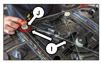
Insert the wire cable (I) around the SST (K) and insert the SST over the pulley (J) as shown.
