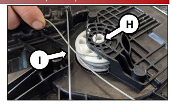
11. Pull the upper wire cable (I) towards the corner pulley (J) as shown.
