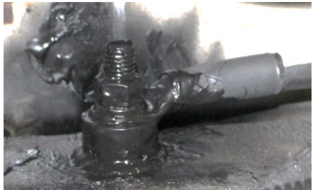
FIGURE 83: GROUND STUD WITH RUBBER COATING
