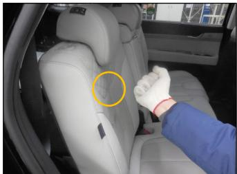
If noise is heard from a rear seat back, carefully remove the affected rear seat (A) using the applicable vehicle shop manual section below:
