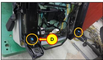
7. Use a heat shrink gun to heat the location pin tubes.
