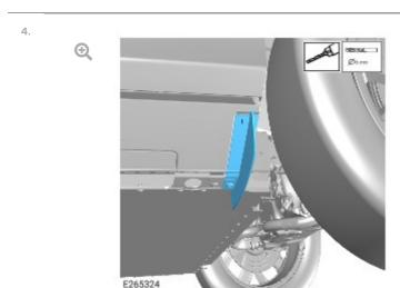
Using a 6 mm drill, create a hole through the left air deflector and the left rocker panel molding in the position marked during step 3.
