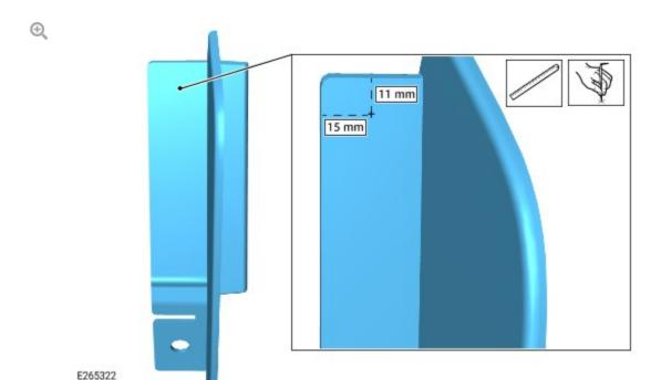
Measure and mark the position on the left air deflector for drilling, as shown in the illustration.
