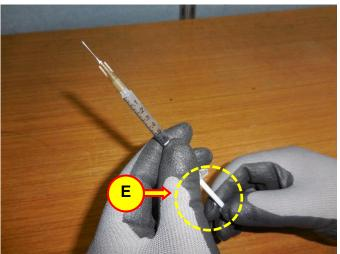
3. Fill the syringe with 0.4ml (D) of Loctite.
