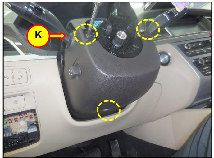
15. Remove the column shaft lower cover (L).
