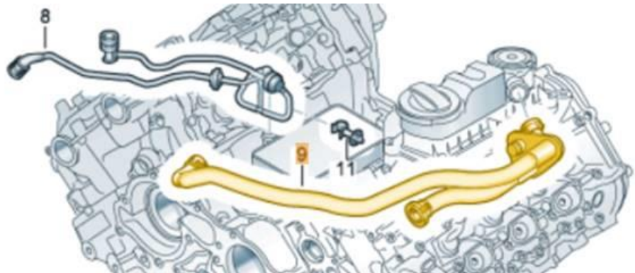
Figure 1. Breather line that needs to be replaced.
