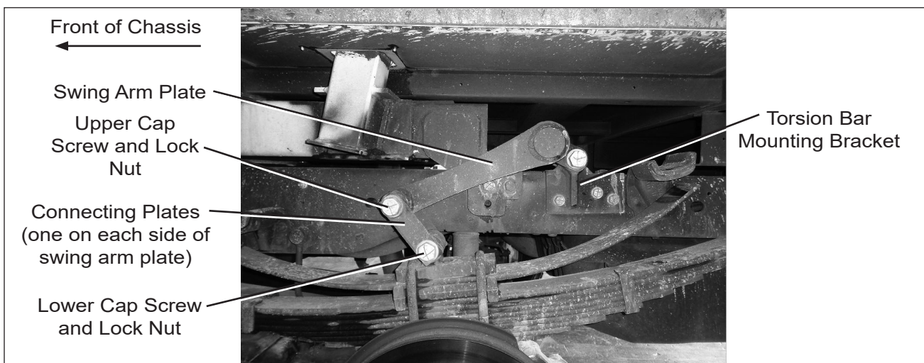
Figure 1 – Street Side Torsion Bar Assembly
