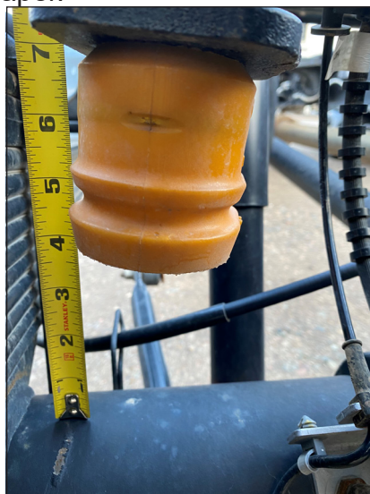
Figure 7 — Measuring for Suspension Travel Number
