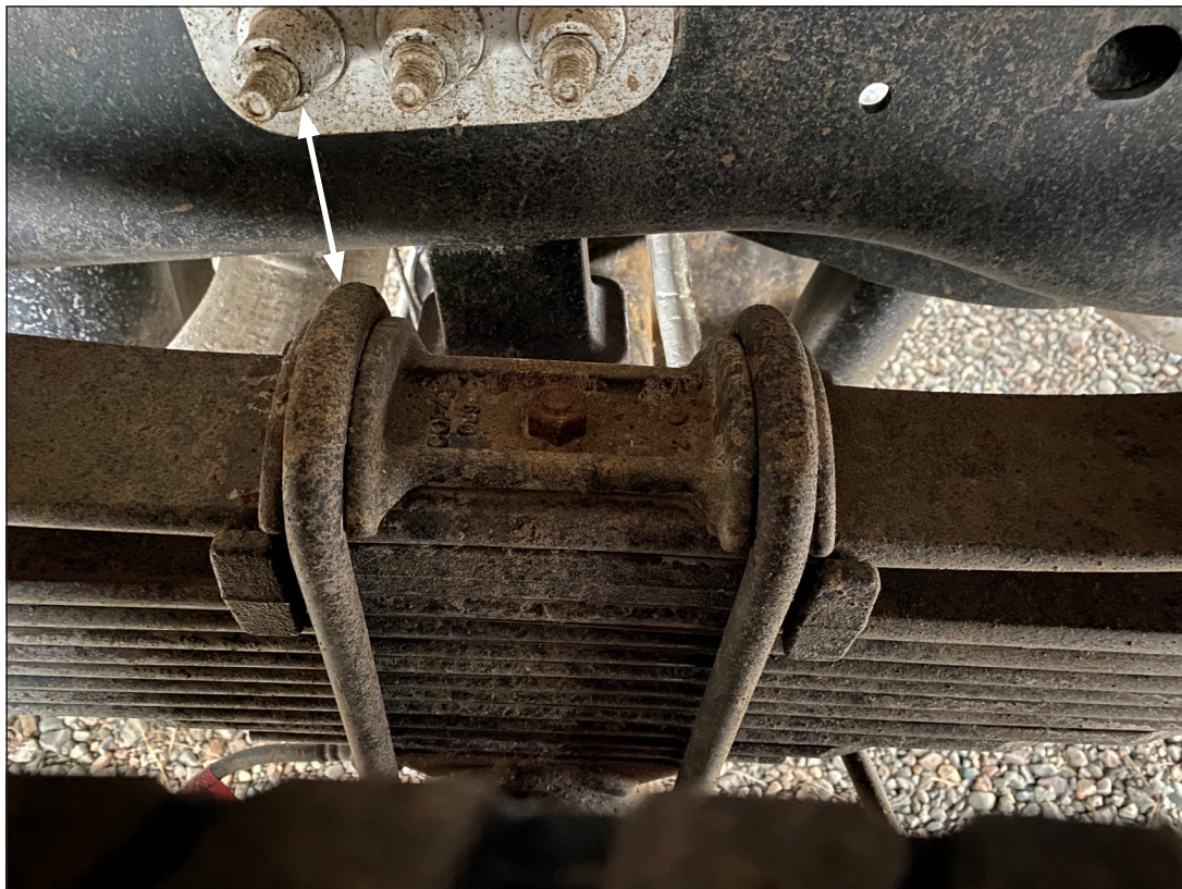
Figure 9 — Identifying Shear Plate Bolt to Measure for Clearance
