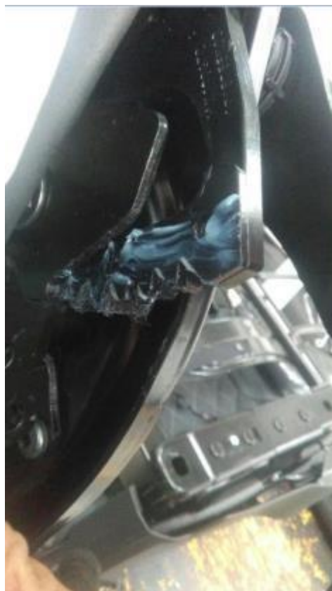
Figure 3. Grease applied to the seat height adjustment toothed segment.
