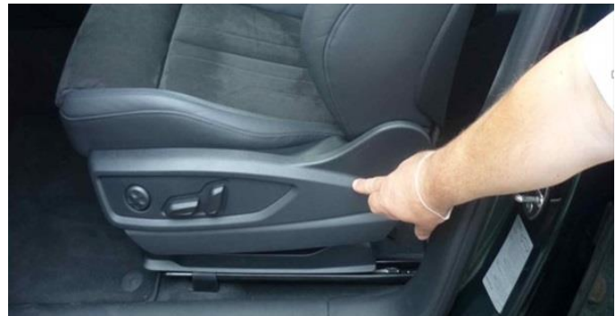
Figure 1. Noise originates from behind the seat frame trim panel near the hinge.
