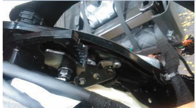
Figure 2. Toothed segment of the seat height adjustment.
