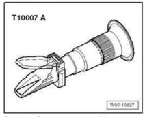
Checking freeze protection of liquid:
