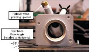
The fuel filler neck must be installed with proper orientation on the body. The neck should be installed with the roll-over valve pointing upward. The bottom edge of the neck mounting flange must be parallel to the ground. See photo for reference.
