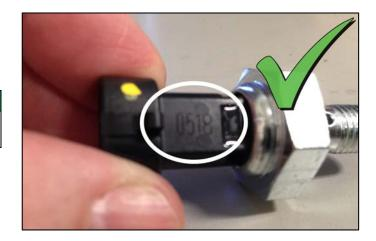
2. Apply a thin layer of lubricant (PN 8560254 provided in kit) to new Stat-O-Seals ①.
