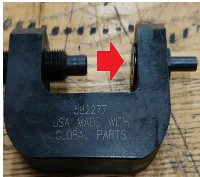
Figure 17. T10172/9 installed in 582277.
