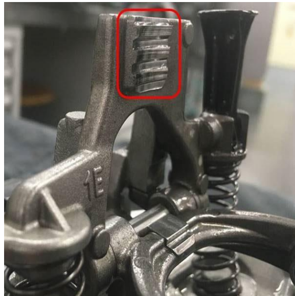
Figure 1. Worn/faulty shift fork.
