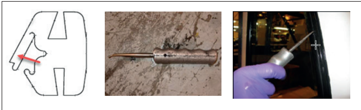
Figure 4 - Unlocking the Rubber Extrusion
