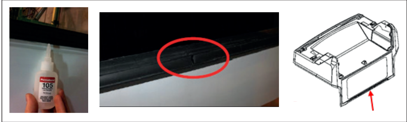
Figure 8 - Usage of Cyanoacrylate Adhesive
