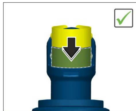
Installing safety clips
