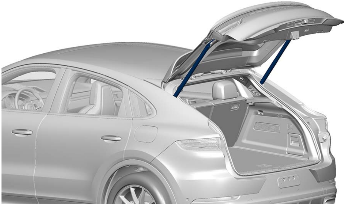
Installation position of ball pins for actuating cylinder
