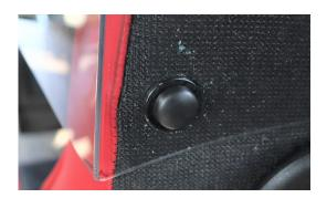
7. **FOR INSTALLATION USING HANDLE:** Secure the partition using a #865358 grab handle, do not over torque the handle screws.
