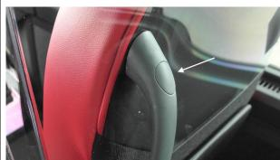
9. <u>Left and right aisle partition</u>: Install decal #7771102 centered on the lower part of the partition (installation with handles shown).
