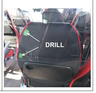
FOR INSTALLATION USING SCREWS: Secure the partition using #508401 washer(s), #504399 cap trim plastic washer(s) and #500337 screw(s). Do not over torque the screws.
