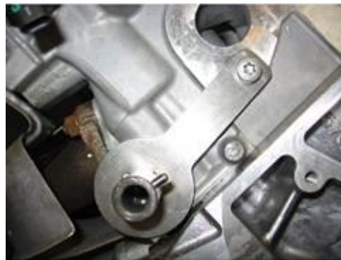
Figure 13. Engine adaptor on bank one.
