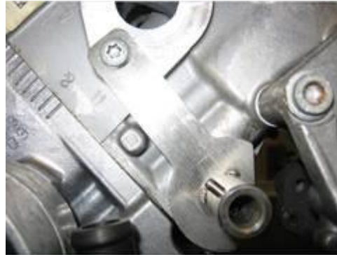
Figure 14. Engine adaptor on bank two.
