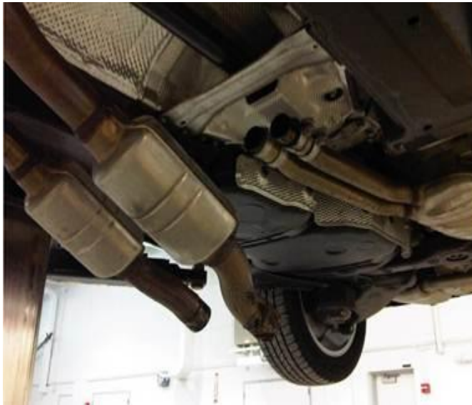
Figure 7. Lowered catalytic converter pipes.
