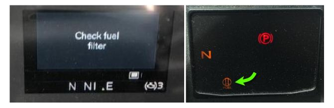
Applicable Vehicles with a main software (MSW) Part Number listed below or newer for the EMS and IC will have the early warning fuel filter restriction message enabled.
