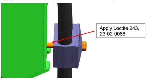
Insert the shim between the mounting bracket and clamp. Re-tighten the bolt and torque it to 80 inch-lbs.
