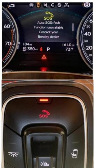
Diagnostic Trouble Code (DTC) U153E00 - Emergency call module and communication unit. Recognition in mobile communications network not possible, stored in Address 75 – Telematics Communication Unit (TCU).
