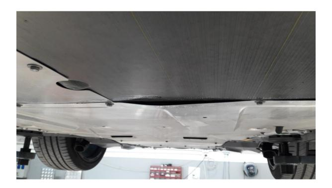
In addition, further inspection is required at the inner engine floor surface as there may be contact between the floor and the fuel tank strap, see picture below.
