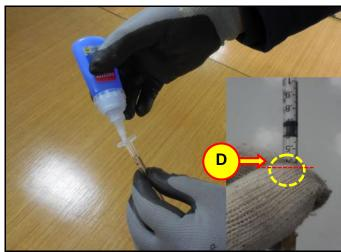
4. Slowly press the plunger (E) inward, to remove any air from the syringe.
