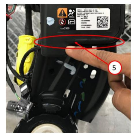
3. Install the first piece of butyl tape by starting it just below the air bag seam (5), as shown below (6). Continue to apply the tape following the contour of the air bag and over the air bag connector (as shown in call outs 3, 7 and 8) making sure to press the tape firmly so there is no looseness in the tape. Only push on the center of the connector. Do not rotate connector and do not apply pressure on the end where the wires exit.
