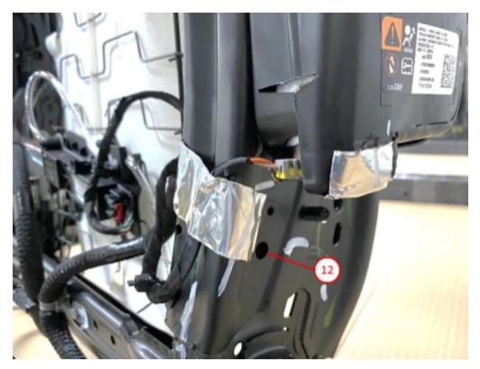
5. Reassemble the seat and use GDS2 to monitor the deployment loop 13 resistance. Verify the resistance is within the normal range and the DTC does not return.
