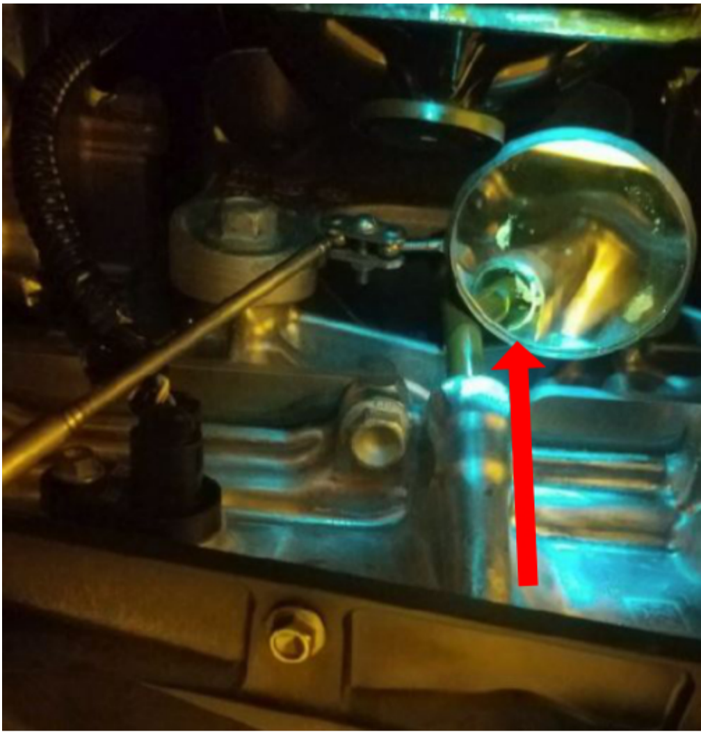
Picture below shows oil leak from composite oil pan sealing surface ( shown with black light and tracer dye)
