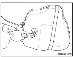
11. After all the fuel has been evacuated, place the tank in an upright position (filler inlet up) and fill the tank with water. Turn off the water when it begins to overflow from the filler neck.
