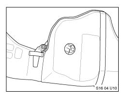
12. With the tank full of water, use an air-powered drill with a  $2\frac{1}{2}$  hole saw. Drill a hole at the bottom side of the tank (on the filler inlet side).
