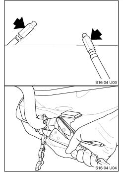
4. Also use the plastic covers from the replacement tank to plug the fuel outlet line and the tank vent line.
