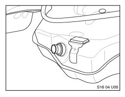
6. Dispose of the stainless steel fill pipe.
