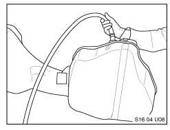
10. Evacuate all fuel remaining in the fuel filter and the outlet line by connecting the fuel caddy to the fuel tank output line.
