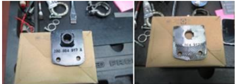
Figure 9. WHT 007 853 reinforcement plates modified.
