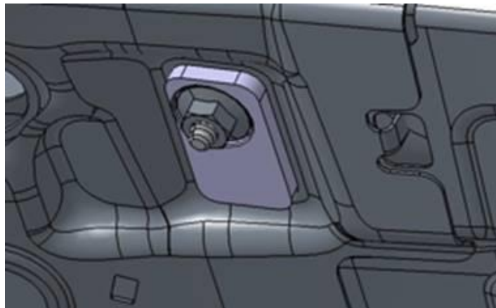
Figure 7. Left side reinforcement plate installation on the Q5.
