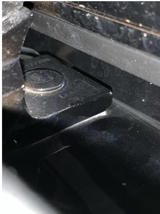
Figure 5. Rear lid hinge mount not flat to the body.
