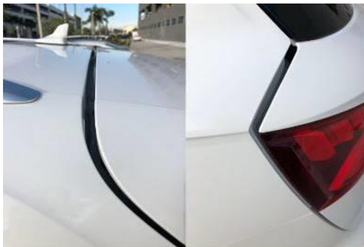
Figure 2. Excessive rear lid gap.
