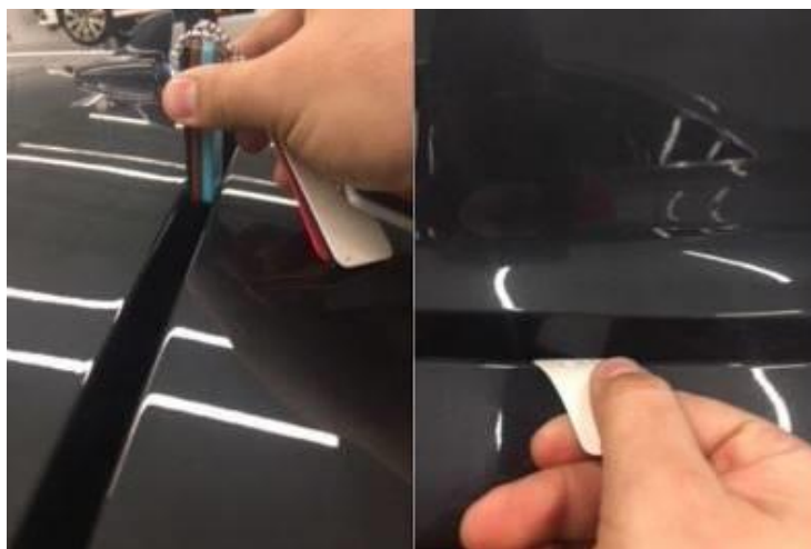
Figure 3. Rear lid alignment out of specification after manually forcing closed an open rear lid.
