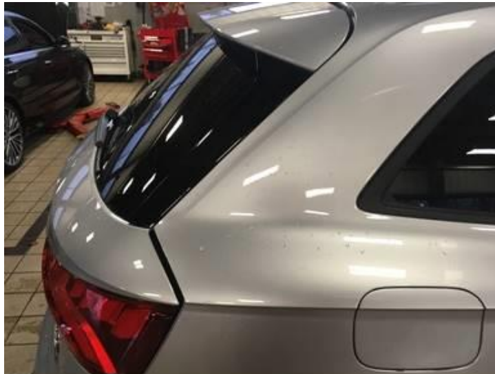
Figure 1. An out of alignment rear lid.
