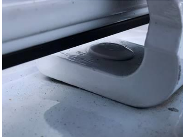
Figure 4. Rear lid hinge mount distorted.
