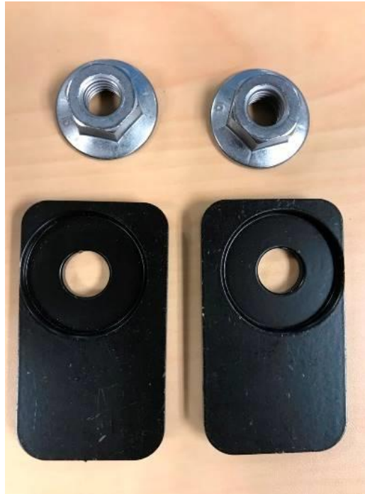
Figure 6. 80A 827 477 (left side) and 80A 827 478 (right side) reinforcement plates and 2 x N 907 988 09 nuts.
