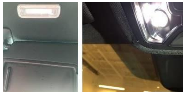
Figure 1. Water intrusion near the headliner.
