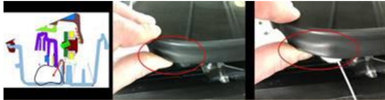
Figure 13. Area of glass panel 'skirt' where bonding agent is to be applied.
