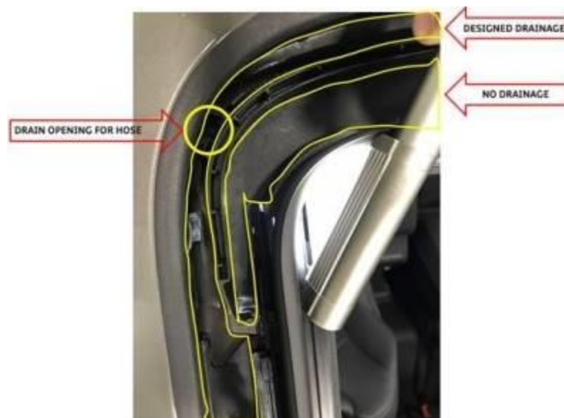
Figure 7. Sunroof water channeling diagram.
