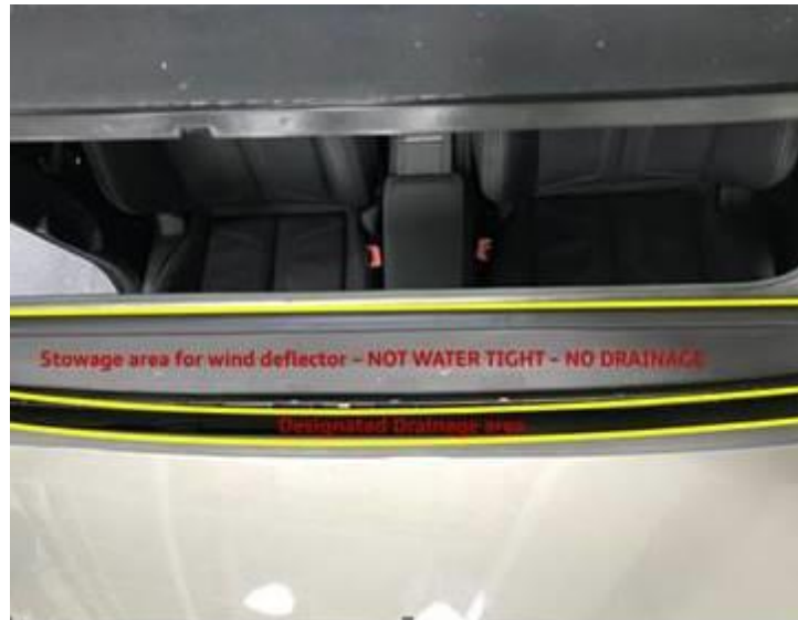
Figure 6. Areas of sunroof opening water elimination capabilities.
