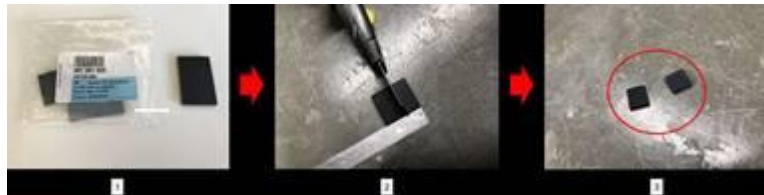
Figure 14. Preparing 2 – 10mm x 10mm pads of 251 201 525 packing.
