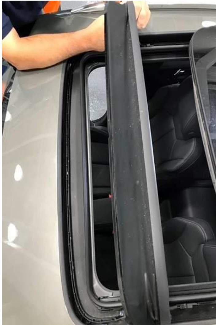
Figure 5. Front sunroof opening with drainage exposed.
