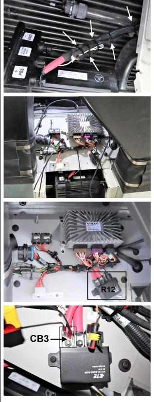
Disconnect the R12 relay AMP type connector (sealed) and connect the two R12 connectors of the ballast box. One end goes to the relay the other end to the disconnected harness.
