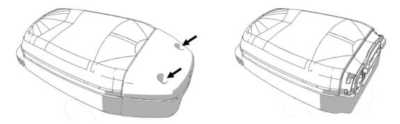
2. On both sides of the camera, insert a small flat blade screwdriver in the opening.
