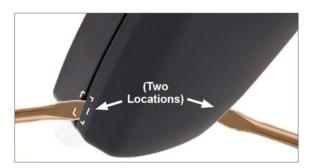
3. Gently prying by moving the screwdriver handles away from the windshield a small amount – push against the retaining clips to release the camera (see image below with the camera hidden to show the mechanism).
