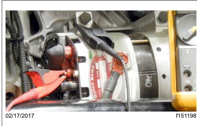
Fig. 14, Clip the DMM positive to the remote sense post and the DMM negative to the alternator body.
