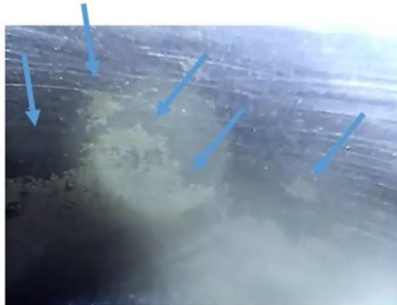
Figure 2. Corrosion marks on cylinder walls (close-up).
