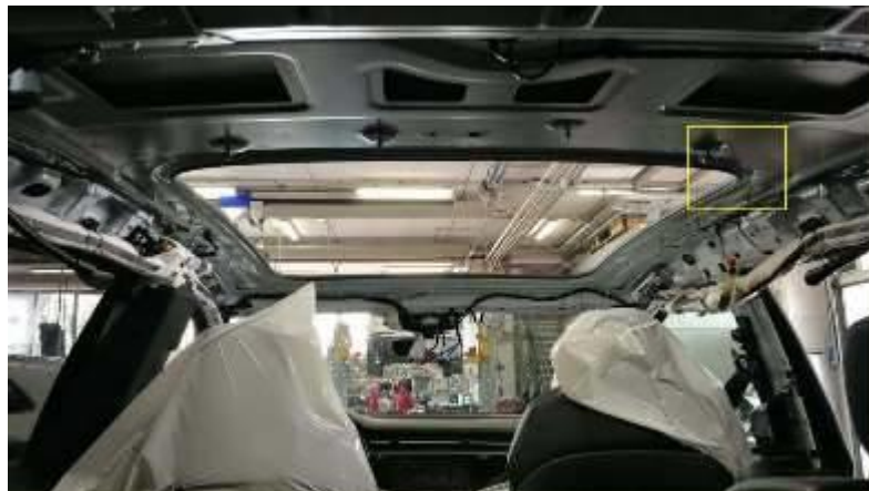
Figure 1. Right rear area of sunroof opening to be reworked.
