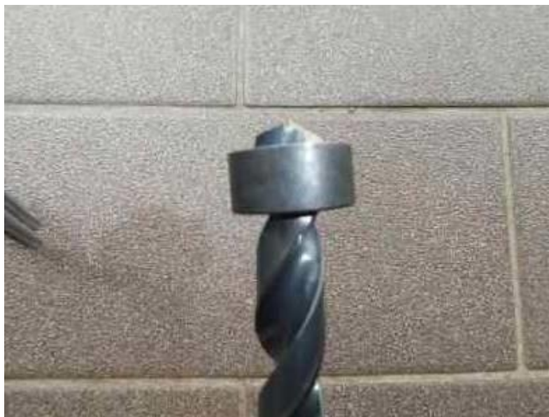
Figure 3. 10 mm drill bit with a depth stop installed.
