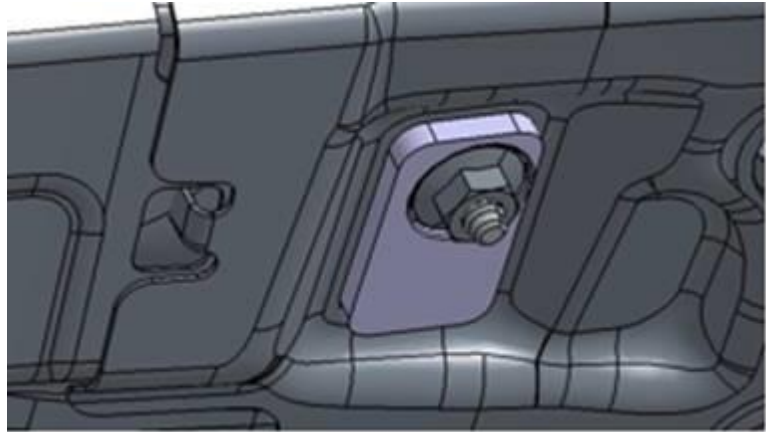
Figure 8. Right side reinforcement plate installation on the Q5.
