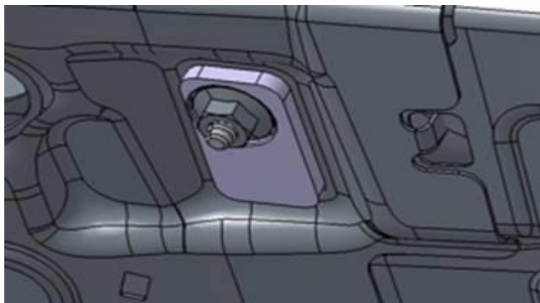
Figure 7. Left side reinforcement plate installation on the Q5.
