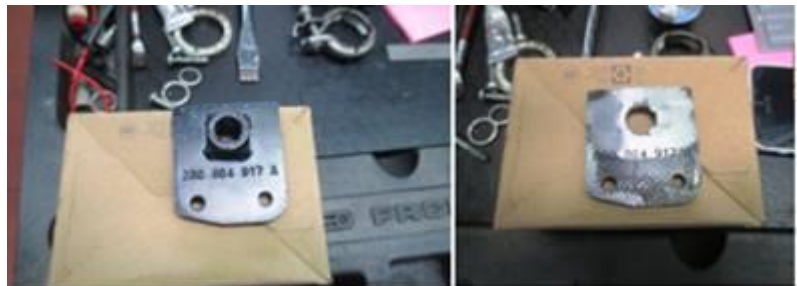
Figure 9. WHT 007 853 reinforcement plates modified.
