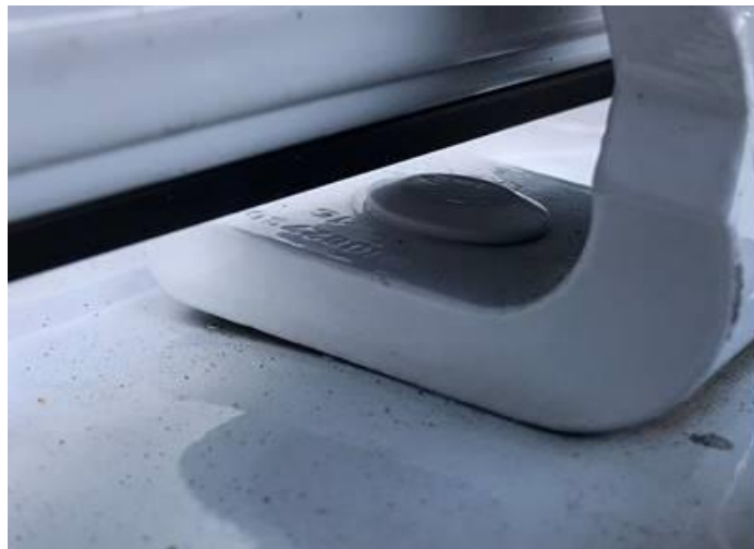
Figure 4. Rear lid hinge mount distorted.
