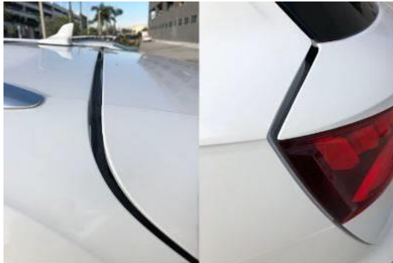
Figure 2. Excessive rear lid gap.
