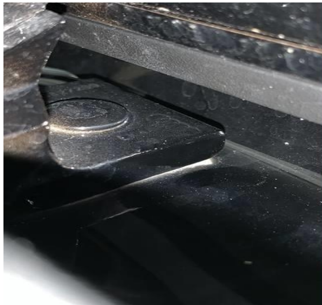
Figure 5. Rear lid hinge mount not flat to the body.
