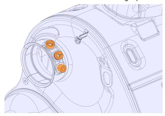
5 Install the new sensor boss and perform the welding.
