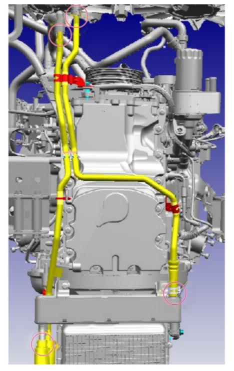
**3.** Transfer the transmission cooler line bracket from the old lines to the new lines. (Figure 2) Figure 2
