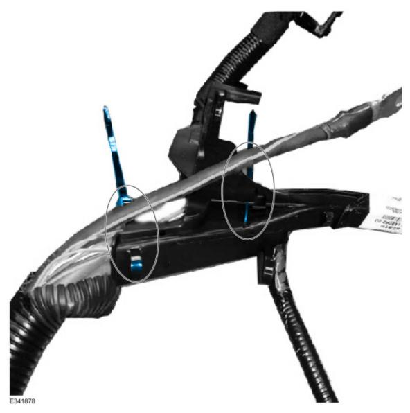
Reroute the engine ground cable outward by pulling it between the 2 red battery cables before the bracket. (Figure 7)
