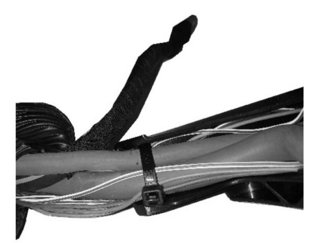
**7.** Remove and discard the 2 tie straps retaining the harness to the harness bracket. (Figure 6) Figure 6
