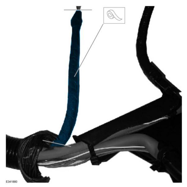
**12.** Using Coroplast tape, wrap approximately 2.5 cm (1 in.) from the ground cable onto the plastic harness guard. (Figure 9)
