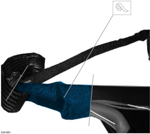
**13.** Reposition the conduit pulled back in Step 6.
