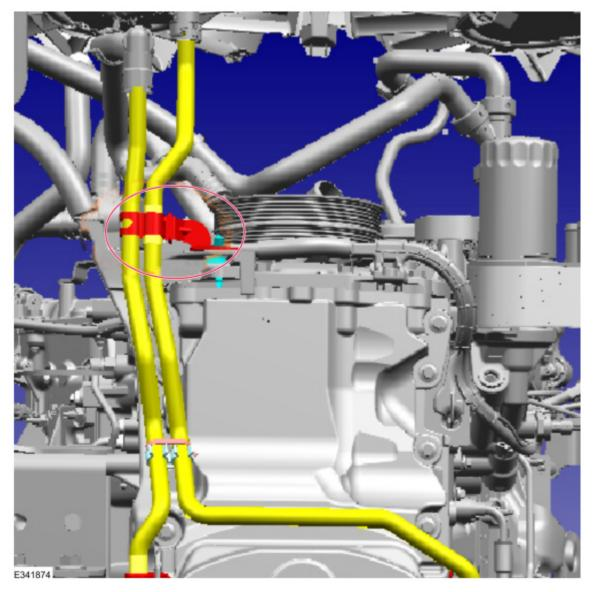
4. Install the new transmission cooler lines.
