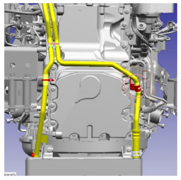
**5.** Remove approximately 15 cm (6 in.) of electrical tape from the engine harness so 5 cm (2 inches) of the conduit is exposed as indicated in Figure 4.
