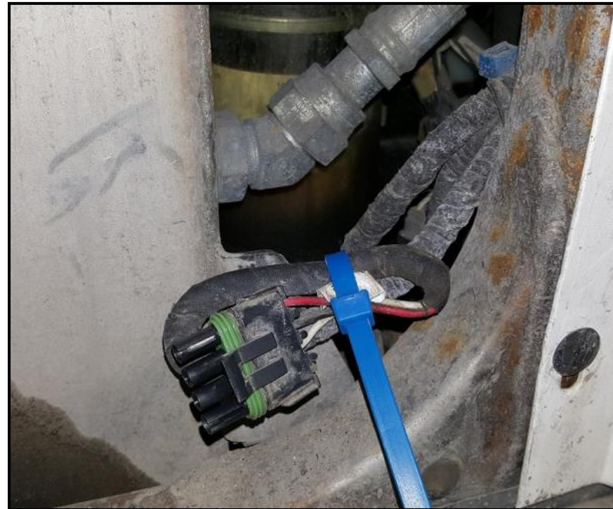
Figure 11– Modified Harness #64 Breakout (+EN-X64H□) Close-Up View
