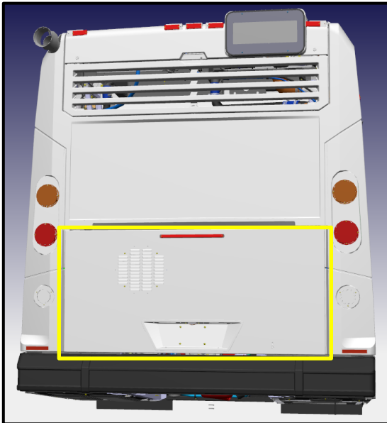
Figure 2 – Rear Door Compartment
