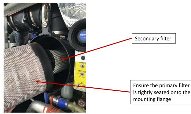
Install the housing cover. Ensure the 4 housing cover clamps are tight and secured.
